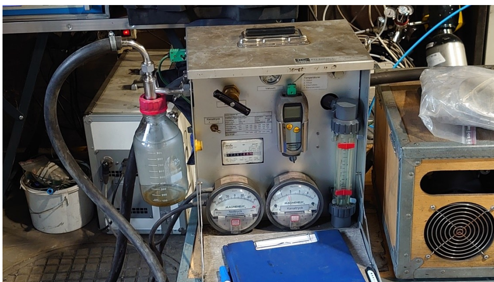
Figure 42 – Ground station of dust measurement equipment.
